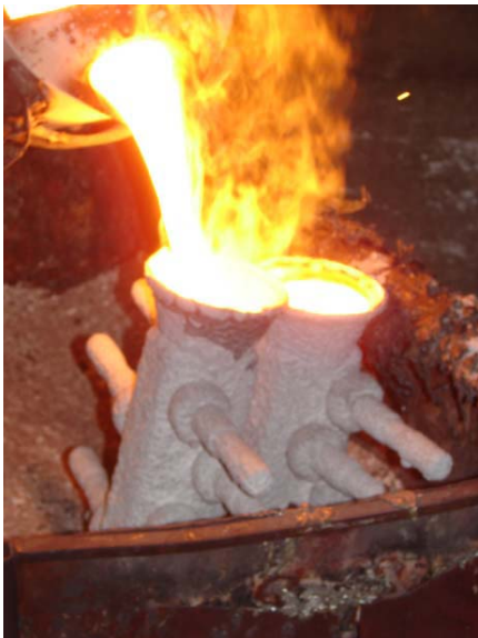
FIGURE 4. Modified shells with 304 stainless steel poured at 3050°F.
