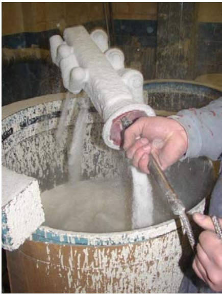
FIGURE 1. Modified shell after being pulled out of the fluidized bed. There is little dust being generated in the bed.
