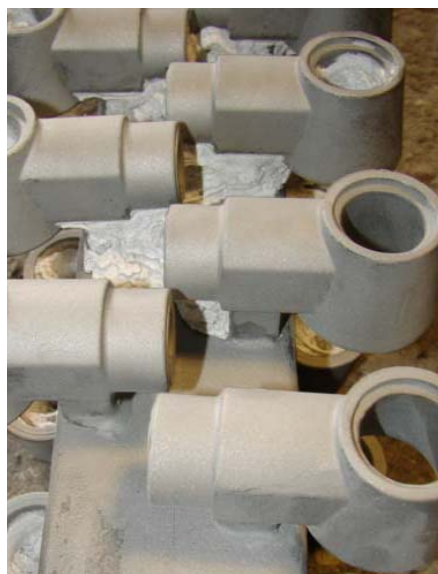
FIGURE 5. Stainless steel casting from a modified shell that has been partially bead blasted to show the surface finish. There is no evidence of burn in or other surface defects.
