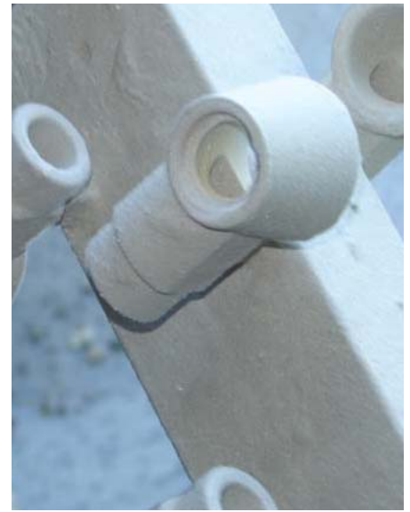
FIGURE 3. Surface of a modified shell made by the litter box method after loose stucco was blown off.
