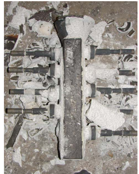
FIGURE 6. Modified shell and stainless steel casting after cooling. The modified shell broke into large pieces during cooling
